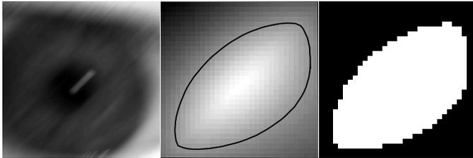
Fig. 1. Illustration of how the motion blur is estimated. **Left:** Center part of the blurred iris image. **Middle:** Point Spread Function (PSF) estimated by way of a blind deconvolution of the blurred iris image. The boundary minimizing the intraclass variance of the 'black' and 'white' pixels (when calculating a binary version of the PSF) is also shown. **Right:** Resulted binary PSF.
