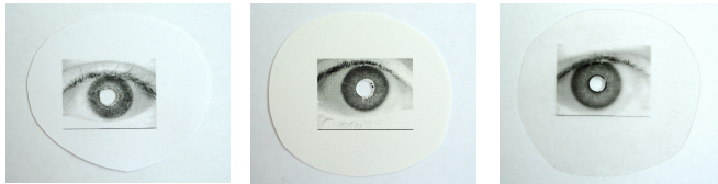
Figure 1. Example printouts on different carriers (from left to right: matt paper, glossy paper and transparent foil) which were used to test the commercial equipment and anti-spoofing methods.
